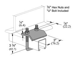
Design Load Each 1000 Lbs (4.4 kN) Use in Pairs Only
