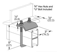
Design Load Each 1000 Lbs (4.4 kN) Use in Pairs Only
